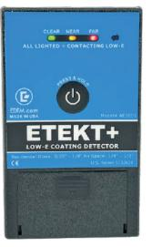
This instrument detects the presence of all electrically conductive coatings in/on a window, including Low-E coatings. Make sure the window is reasonably clean before testing. The "FAR" and "CLEAR" indicators are dependent on the window being within the thickness specifications listed above. If in doubt about the thickness of the window being tested, always test both sides of the window and look for the side that yields the "NEAR" indication. The "NEAR" indication works for any glass thickness.
