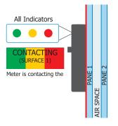
When the ETEKT+ is in direct contact with a LOW-E coating the GREEN, YELLOW and RED indicators will all be lighted.
